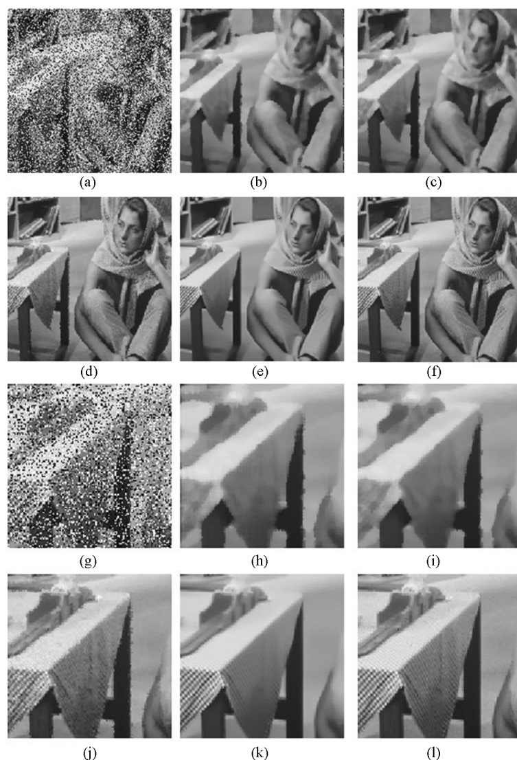
Fig.4. (a) Image “Barbara” corrupted by salt-pepper noise with 30% level. Restored images by (b) MF ( 7 \times 7 ) with PSNR = 22.28 dB. (c) WMF ( 7 \times 7 ) with PSNR = 25.65 dB. (d) AMF ( 7 \times 7 ) with PSNR = 29.46 dB. (e) UNLM with PSNR = 32.81 dB. (f) NLMED with PSNR = 35.29 dB. (g)~(l) are their corresponding closeups.
