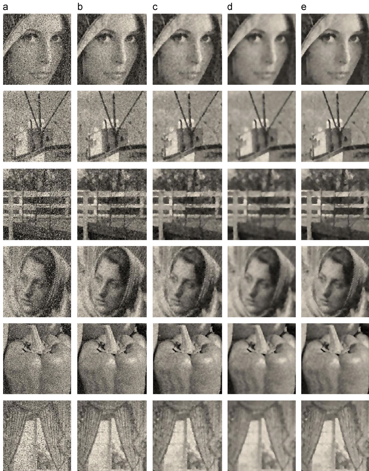
Fig. 5. Closer investigations of the three tested images corrupted by the mixed noise with r=0.2 and \sigma=25 . From left to right: (a) the noisy data, (b) restored by SD-ROM [27], (c) restored by Trilateral [9], (d) restored by MNF [10] and (e) restored by our multi-kernel method.
