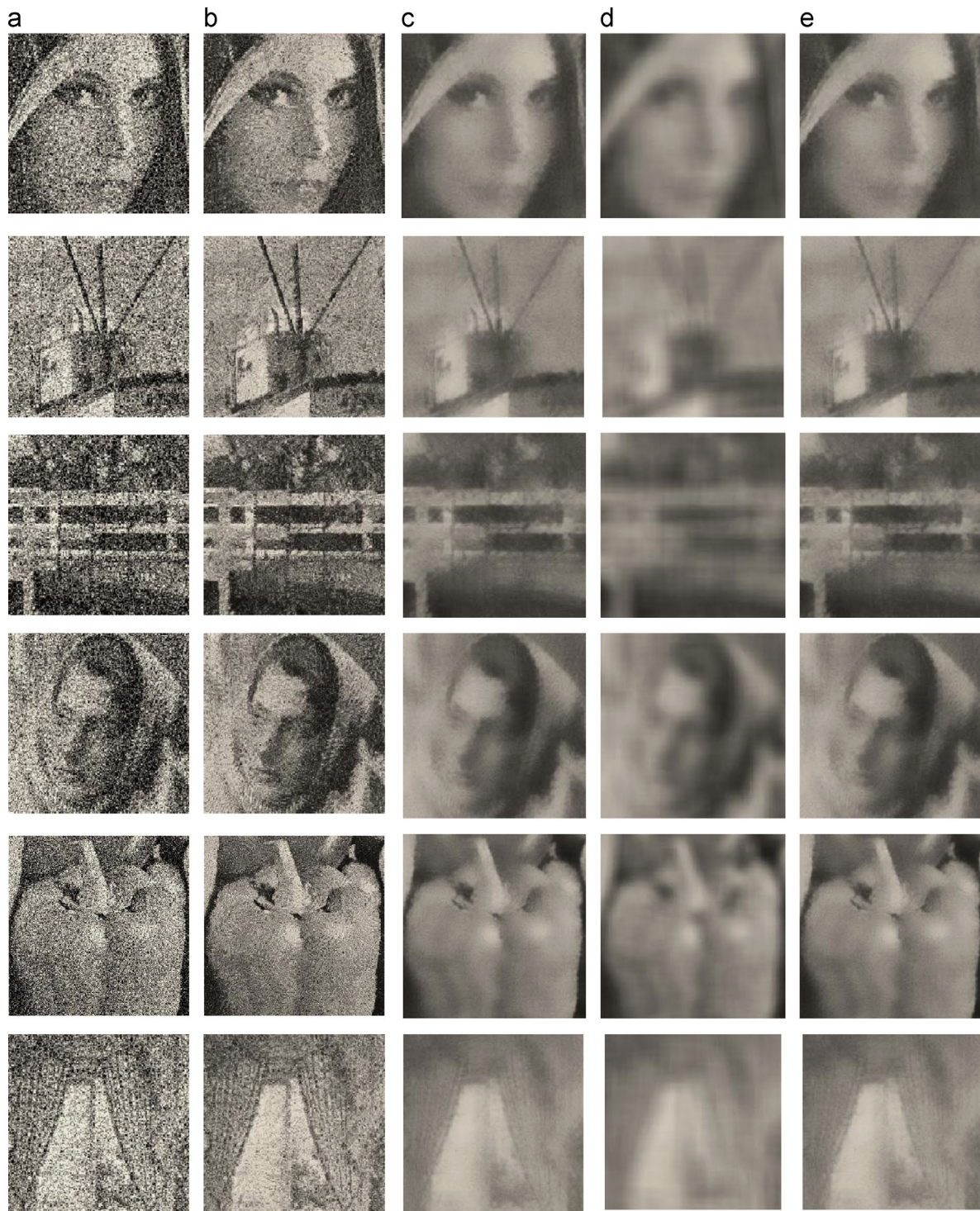
Fig. 4. Closer investigations of the six tested images corrupted by Gaussian noise with \sigma=70 . From left to right: (a) the noisy data, (b–d) restored by the single kernel methods with h^2=10\sigma (NLM) [4], 100\sigma , 1000\sigma respectively, and (e) restored by our multi-kernel method.
