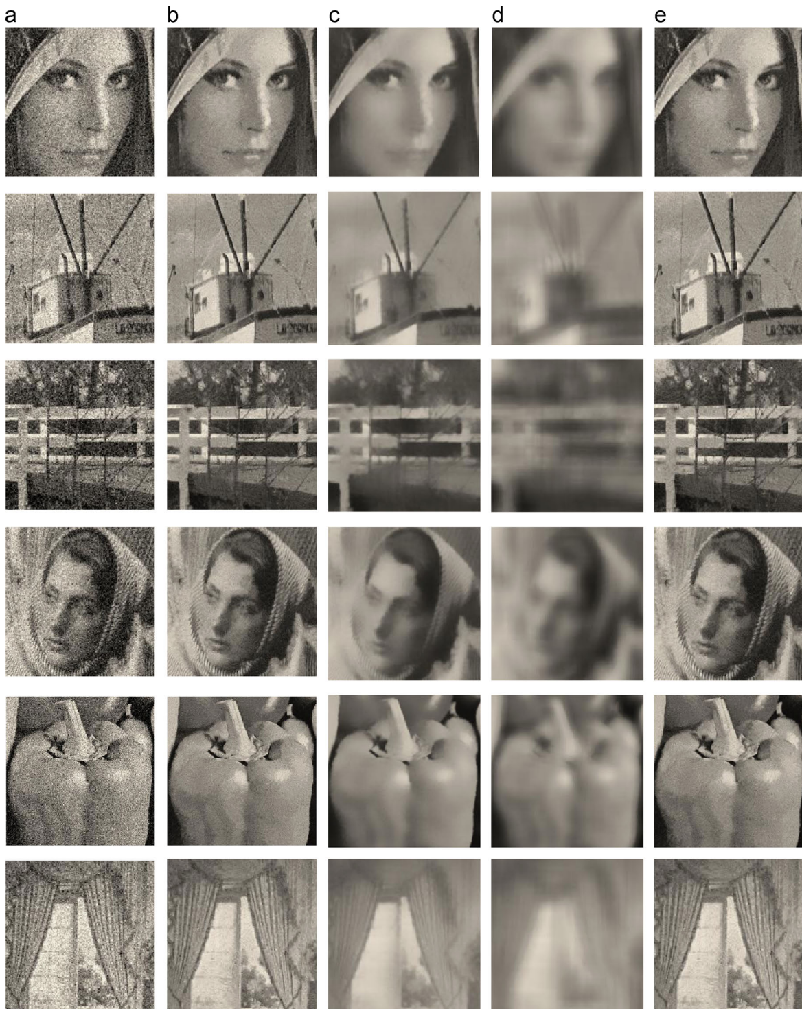
Fig. 3. Closer investigations of the six tested images corrupted by Gaussian noise with \sigma=30 . From left to right: (a) the noisy data, (b–d) restored by the single kernel methods with h^2=10\sigma (NLM)[4], 100\sigma , 1000\sigma respectively, and (e) restored by our multi-kernel method.
