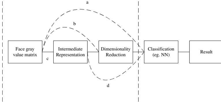
Fig. 1. Illustration of the appearance-based face recognition.
