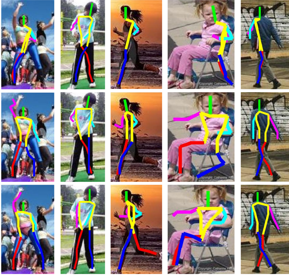
Fig. 3. Visualization of various methods for human parsing on the still web image data set. From top to bottom, each row shows the results yielded by the baseline model [28], our method with action-specific \ pose-specific experts, respectively.
