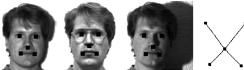
Fig. 10. Three examples from the training set showing the locations of the labeled features and the structure of the learned pictorial model [25].
