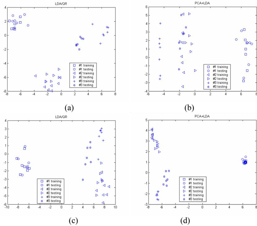
**Fig. 3.** Two dimensional display of samples from three classes respectively by LDA/QR and PCA+LDA, where pictures in the same row correspond to the samples from same three classes: (a) and (b) illustrate the case that PCA+LDA classifies some testing samples wrongly while LDA/QR discriminates the three classes correctly, (c) and (d) show the case that LDA/QR some testing samples wrongly while PCA+LDA discriminates correctly.
