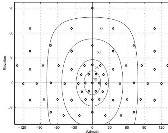
**Fig. 4.** The azimuth and elevation of the 64 strobes. Each annulus contains the positions of the strobes corresponding to the images of each illumination subset-Subset 1 ( $12^\circ$ ), Subset 2 ( $25^\circ$ ), Subset 3 ( $50^\circ$ ), Subset 4 ( $77^\circ$ ) Subset 5 (outer annulus) [6].
