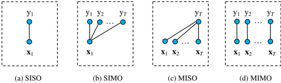
**Fig. 1.** Illustration on four different learning problems. Here, each edge represents a model, and the nodes  $x_j$  and  $y_j$  denote the imaging data (input) and clinical scores (output) at  $j$ -th time-point, respectively.
