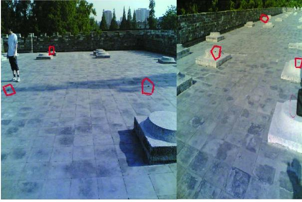
Fig. 1. Network deployment of fire alarming WSN of ancient city wall.
